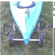
2. Lift the kayak by the stern and place it on top of the cart. The kayak hull does not have to be resting on the bottom of the V. Side hull contact on the rubberized sides will work file.
