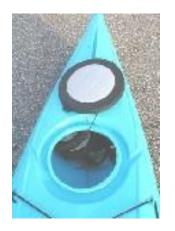
6. The Packaway cart will fit through openings as small as an 8" round hatch by folding the arms down and taking the wheels off. Simply pull the clevis pins to remove the wheels. Note: Replace the clevis pins in the axle so you don't lose them. If lost, clevis pins can be found at most hardware stores.
