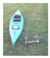
1. Place the cart next to the stern (back) of the kayak as shown. Have the control arms pointing at the front tip of the kayak, so the cart and boat are aligned when you lift the boat onto the cart. Generally, the best fit is with the hull down as far as possible in the V of the cart. Very wide kayaks may rest high in the V.
