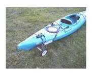
4. Place the hook in the center of the cockpit coaming and snug the control straps firmly and evenly. Snugging each side up 3" or 4" at a time makes this easy. They should be snug but not too tight.
