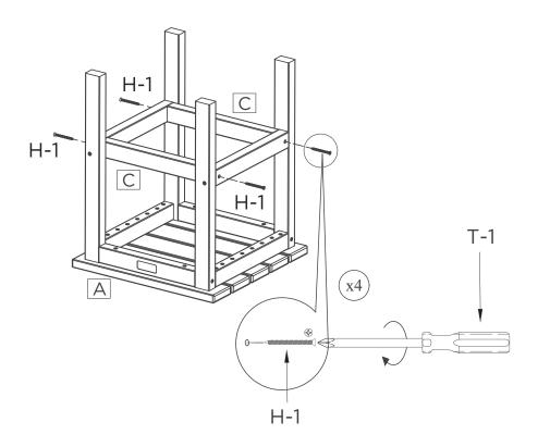
Place the Brace (C) in place and fasten using two Phillips Head Screws (H-1) and a Phillips Screwdriver (T-1). Repeat for the other Brace (C). Fully tighten all hardware from this step and all previous steps. DO NOT OVER-TIGHTEN.
