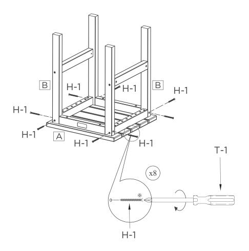
Place the Tabletop (A) upside down on a flat surface. Install the first Leg Assembly (B) onto the tabletop. Fasten using four Phillips Head Screws (H-1) and a Phillips Screwdriver (T-1). Repeat for the other Leg Assembly (B). Do not yet fully tighten.
