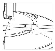
Note location of fire pit support bracket when installed correctly.
