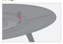
**O5.** After pushing down, press the **cap** in toward the perforated grate.
